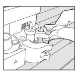
1. Open Clamp B and remove blade housing.
