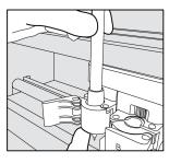
3. Hold Clamp A up with fingers while pushing pen down into clamp until arrow on pen disappears.
