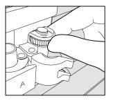
Place blade housing in Clamp B, ensuring that housing is seated on the top surface of the clamp. For Rotary and Knife blades, make sure the gears fit together.
