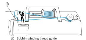
Slide the bobbin winder shaft to the left, and then remove the bobbin from the shaft.
