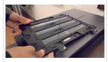
Lift the top cover of the scanner. Remove the white tray on the top by sliding it up and out. Put the tray of negatives on the platen with the white arrows face up on the right.
